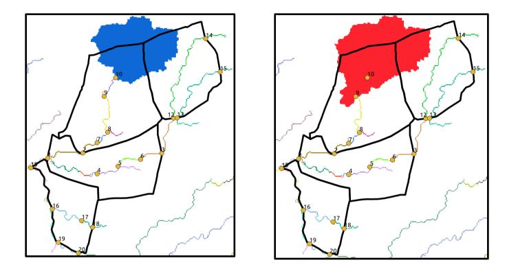
Now, the differential watershed for point 9 is the amount of water accumulating at point 9 and is not part of the watershed for point 10. The below area marked in green represents the differential watershed for point 9. Say "X" amount of water is available in the watershed for point 10 and "Y" amount of water is available in the watershed for point 9, then the differential watershed for point 9 will comprise of "Y-X" amount of water.
