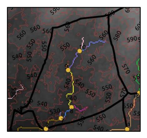
In the above figure, it can be seen that for point 7 the elevation value from contour is 530 and for point 10 it is 550 then it can be concluded that the water is flowing from point 10 to point 7. Similarly, for other points, the contour values will be useful to derive the flow.
